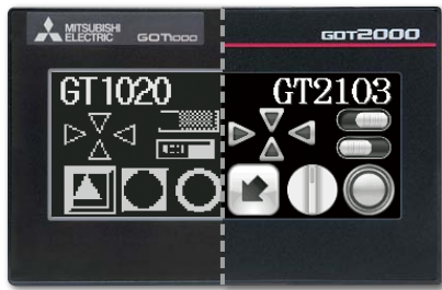
GT1020 Monochrome (black/white) STN LCD GT2103 Monochrome TFT LCD with 32 gray scales
