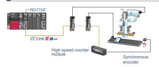
The operation timing between multiple slave units is aligned since the synchronous communication compatible slave devices operate simultaneously with the operation cycle of the Simple Motion module.
