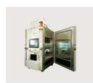
Equipment for highly accelerated life tests (HALT)
